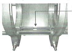
Take care that it lies in the zone of the diminution of the tear-off bar, if required displace the shaft.
