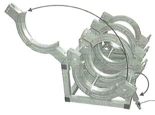
Spindle with lock nut and washer, swung out
