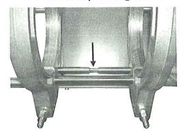
There is a tear-off bar mounted between the flexible and the fixed clamping rings on the basic machine. It prevents the heating element from sticking to the heated-up pipe ends.
