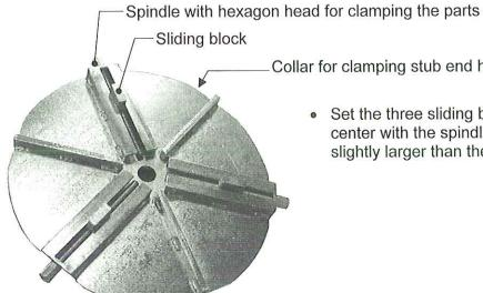
Collar for clamping stub end holder into clamping tool
